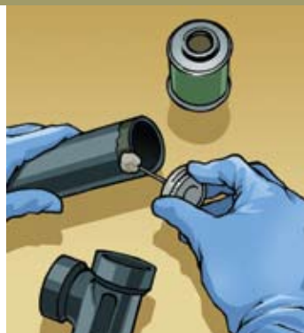
Gluing of ABS and PVC pipes
