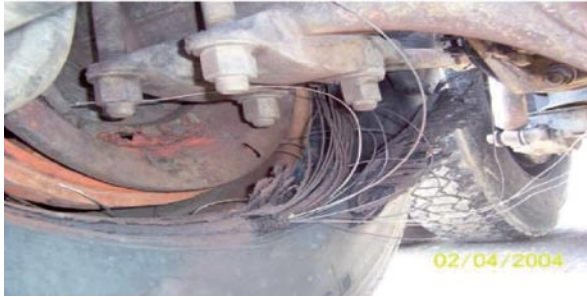
Photo no. 1: Example of a tire that burst following brake overheating (locked brakes).
