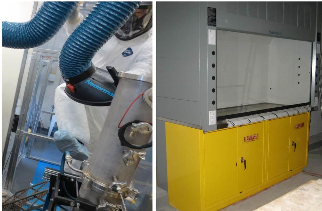
**Figure A2: Source capture system and fume hood**
