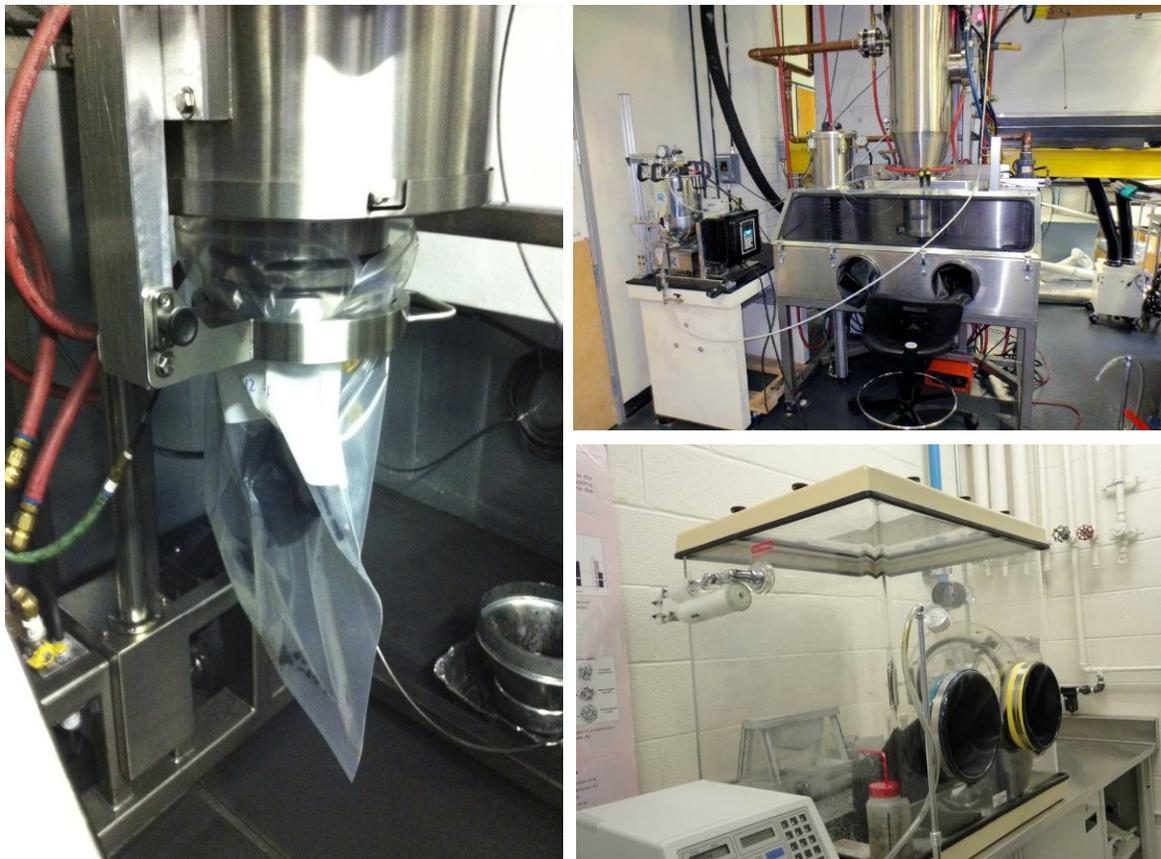
**Figure A3. At-source containment systems**
