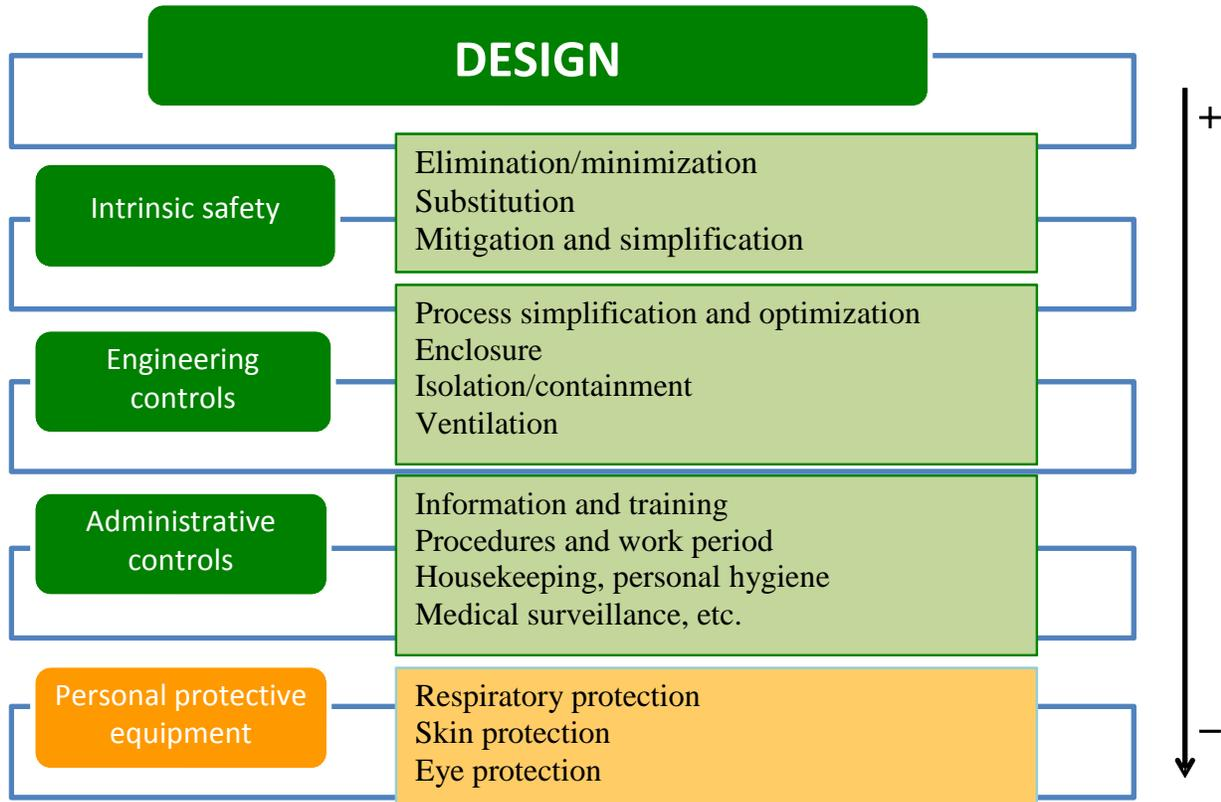
**Figure 10: Hierarchy of nanomaterial exposure controls**
