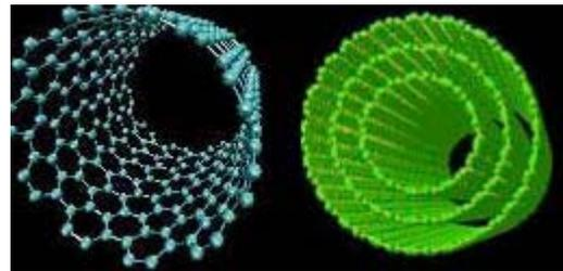
**Figure 1: Schematic illustration of a single-walled carbon nanotube (SWCNT) and a multiwalled carbon nanotube (MWCNT)**
