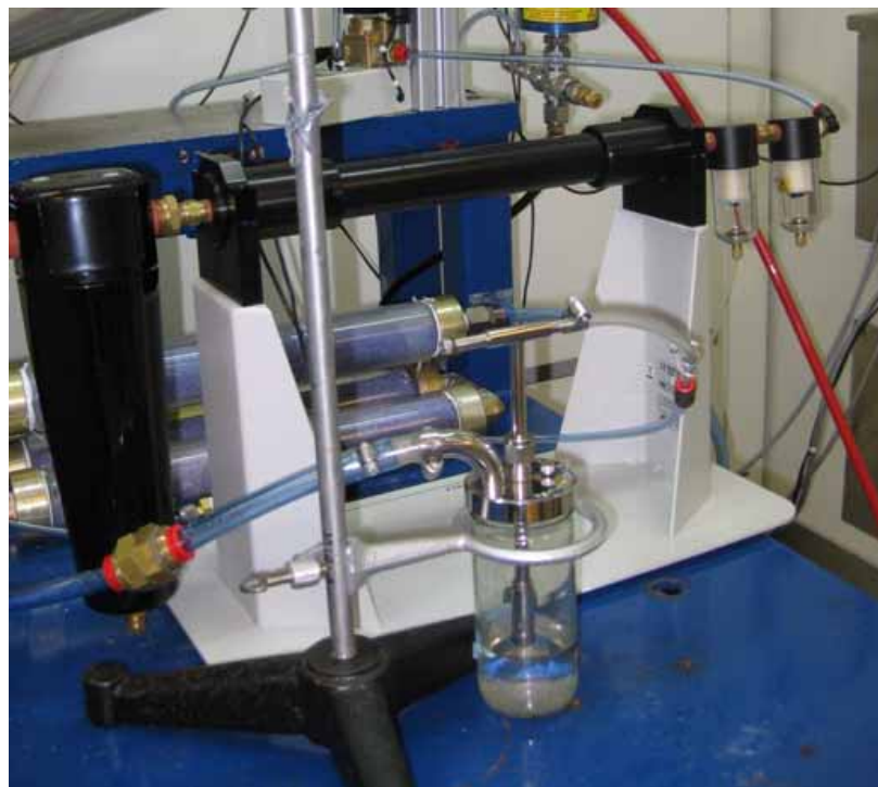
Figure 2-9: Photograph of the filtered air supply (Model 3074, TSI Inc.) connected with six-Jet Collision Nebulizer.
