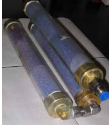
Figure 2-10: The silica gel drying system.
