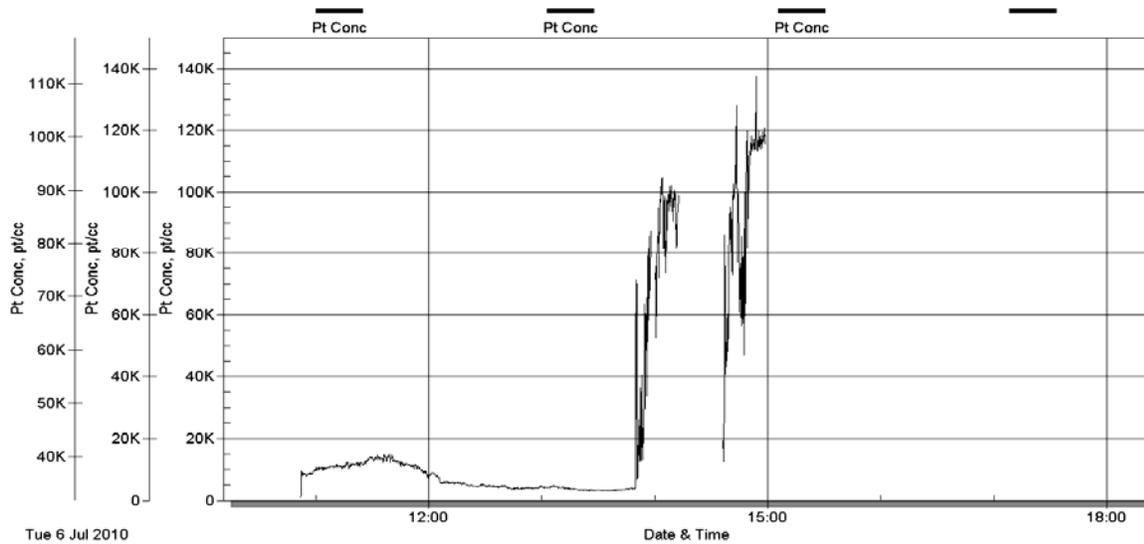
**Figure 16 – Particle concentrations measured in the processing room**
