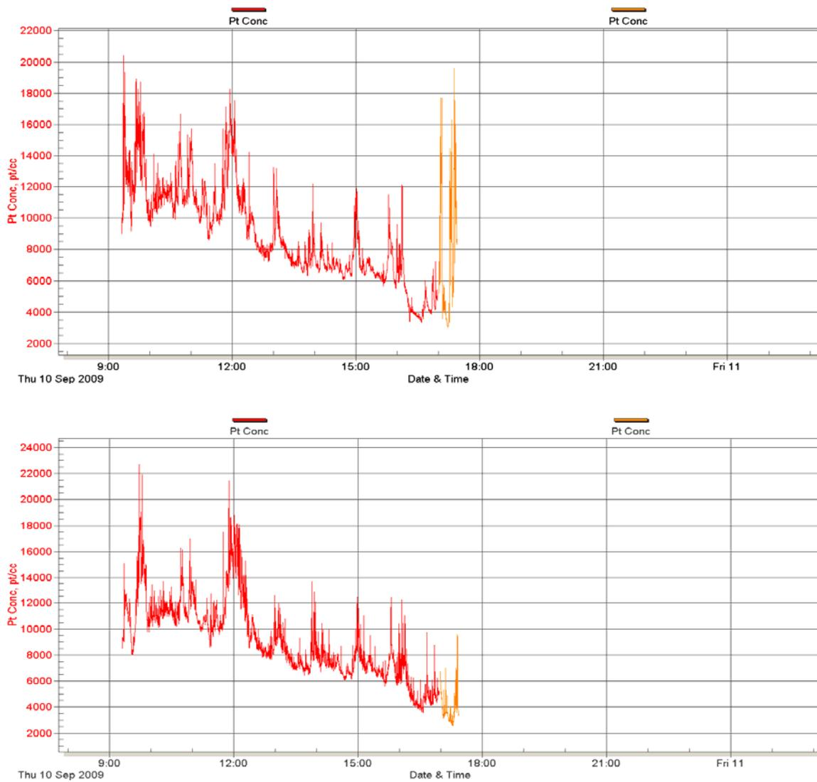
**Figure 19 – Profiles of particle concentrations measured with P-Trak particle counters on the 3<sup>rd</sup> day of sampling near the mill (i) and 3 metres from the mill (ii) (Laboratory A)**
