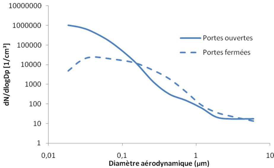
**Figure 8 - Comparison of particle granulometric distributions based on opening of the potroom doors in the prebaked anode process**
