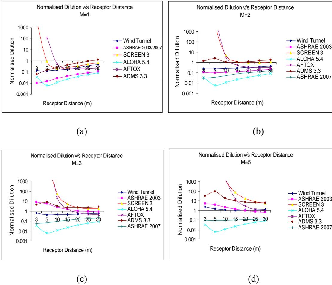
Figure 5.13 Normalised dilution versus receptor distance for a stack height of one metre; low-rise building with roof top structure
