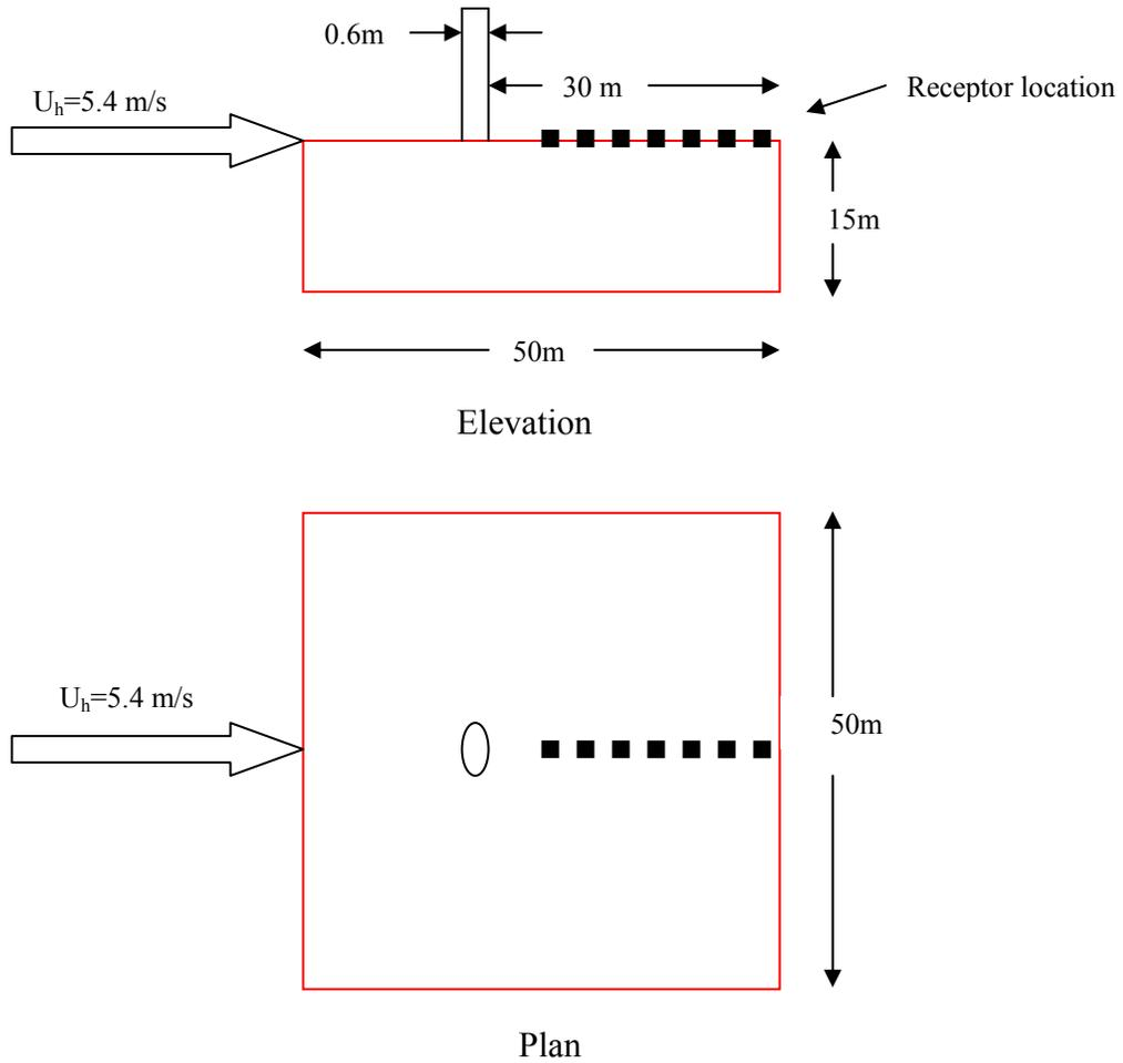
Figure 5.1 Low-rise building with stack and receptor location
