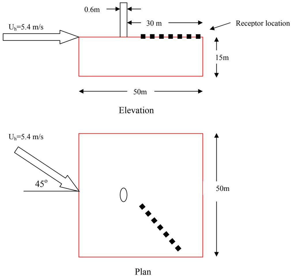
Figure 5.17 Low-rise building with wind direction at 45 degrees
