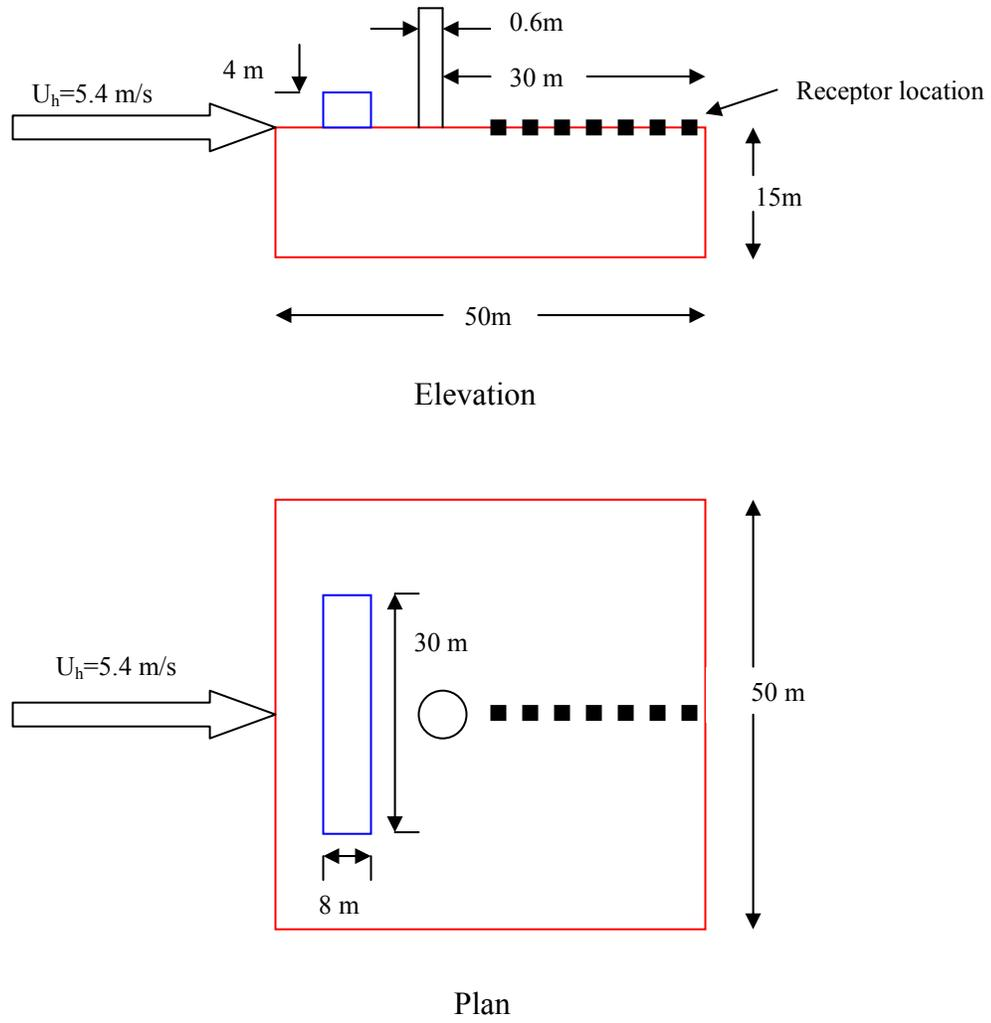
Figure 5.12 Low-rise building with roof top structure
