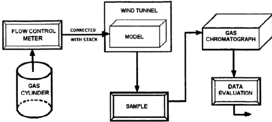
Figure 4.5 Tracer Gas Experiment System (from Gupta, 2008)
