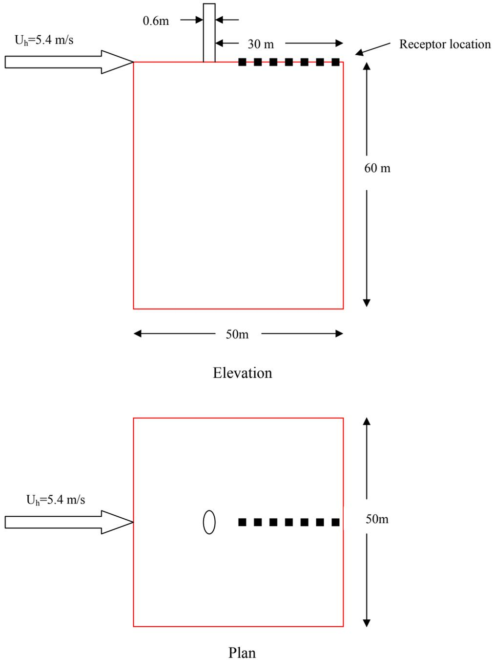
Figure 5.7 High-rise building with stack and receptor location
