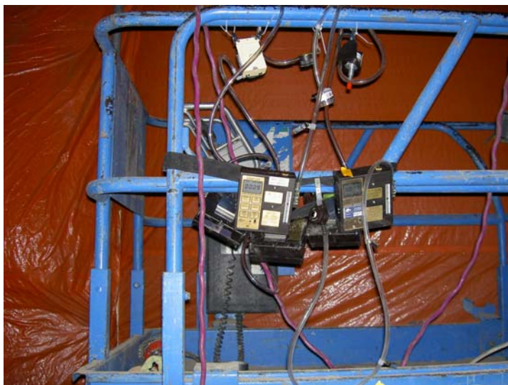
Figure 14: Ambient air sampling with sampling devices attached to the lift
