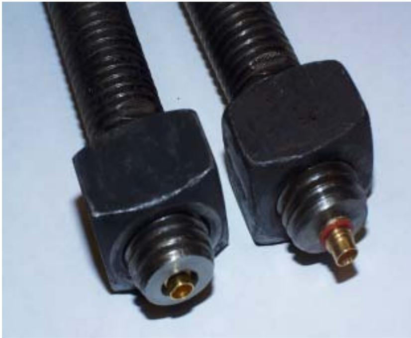
Figure 33 New (left) and initial (right) placement of device connector
