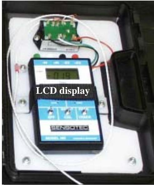
Figure 9: Readout unit
