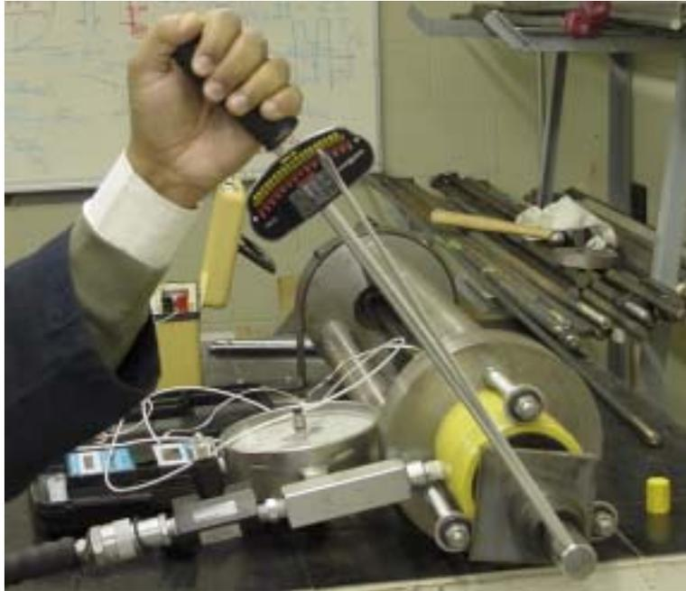
Figure 14: Axial loading of the bolt using a torque wrench
