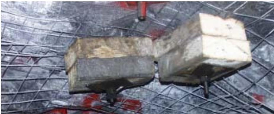
Figure 28: Timber blocks shield the instrumented bolts from subsequent blasting effects
