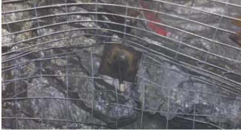
Figure 23: SAFEBOLT-Instrumented 5/8" Mechanical rockbolt
