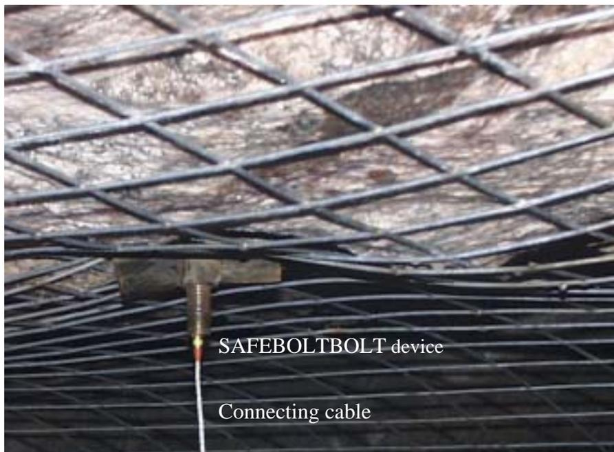
Figure 20: Measuring axial load using SAFEBOLT system at Niobec mine
