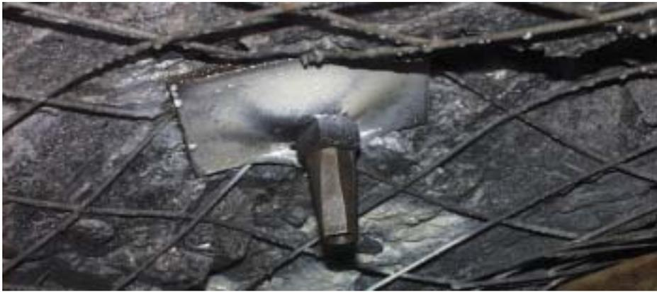
Figure 27: Protection of the SAFEBOLT device using the nut of the expansion shell
