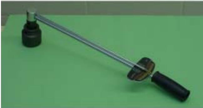
b) Toque wrench used for the test
