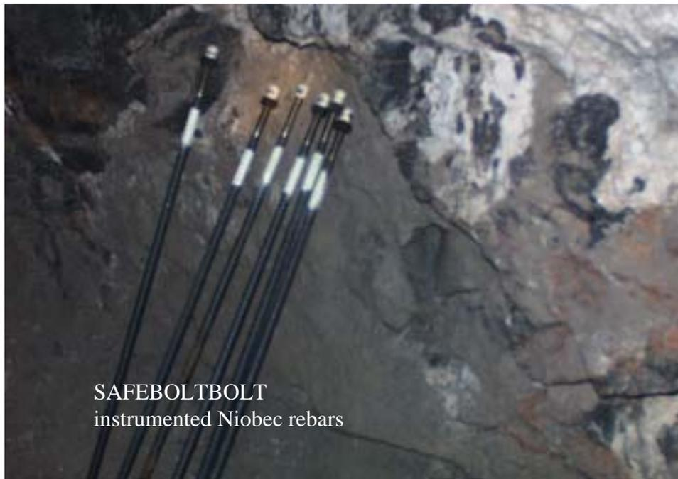
Figure 19: SAFEBOLT instrumented before installation
